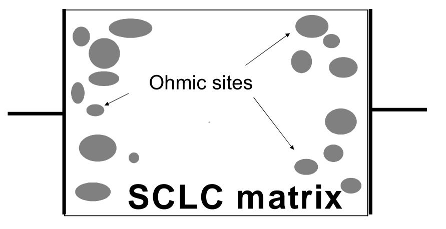
Trap-filling regime: the system can be viewed as a disordered matrix with embedded insulating and ohmic sites forming intricate paths.
