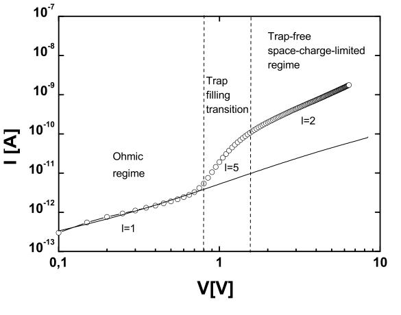
Ideal insulators: transport occurs via carrier injection, as in the vacuum tube. The I-V is quadratic over all the voltage range (Mott-Gurney Law)
