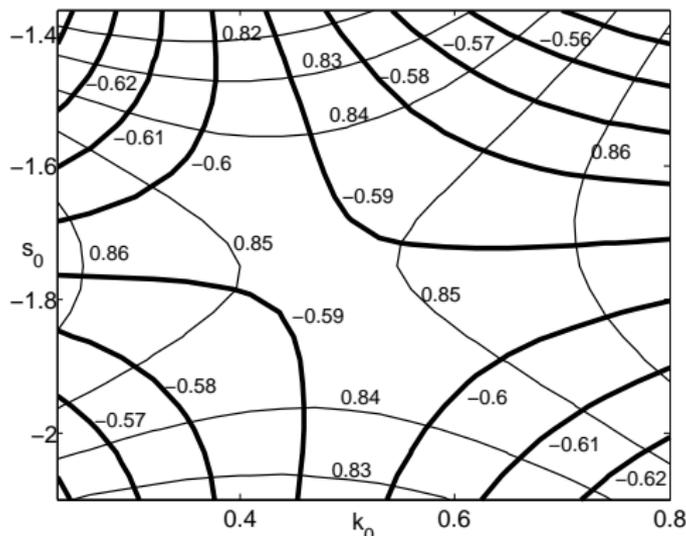
$Re = 35, x = 4$ . Level curves,  $\omega_0 = \text{const}$  (thin curves),  $r_0 = \text{const}$  (thick curves).
