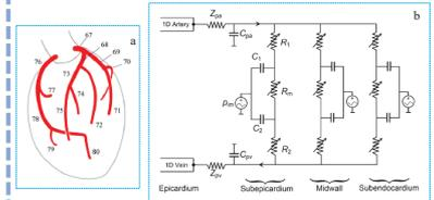
Fig.2: (a) 1D Left-coronary arteries included in the model. (b) Representation of the 0D model closing each coronary artery. Both figures are extracted from [5].
