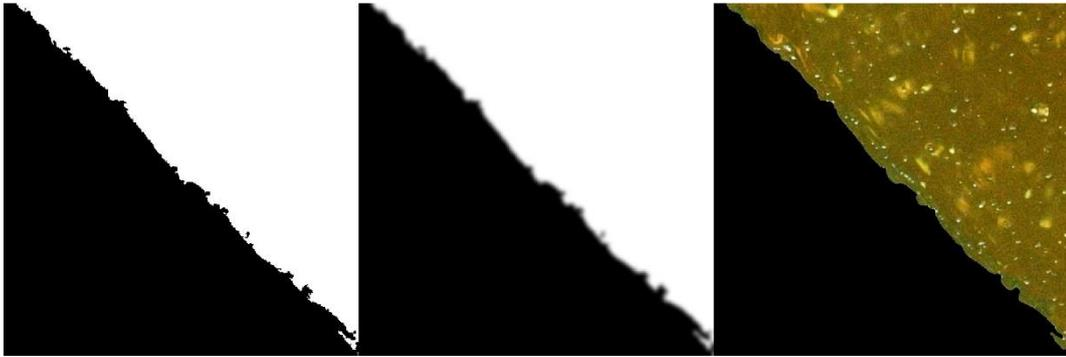
*Figure 74 Three main processes (optimised for the lower surface) to detect the body in the photo. On the left: binarization of the photo obtained by the subtraction of the blue channel from the red channel. In the middle: Gaussian filter applied to the previous photo. On the right: Binarization of the photo in the middle and multiplication by the original photo.*
