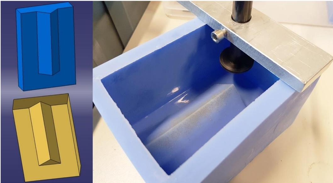
*Figure 58 “V-shaped” base mould.*
