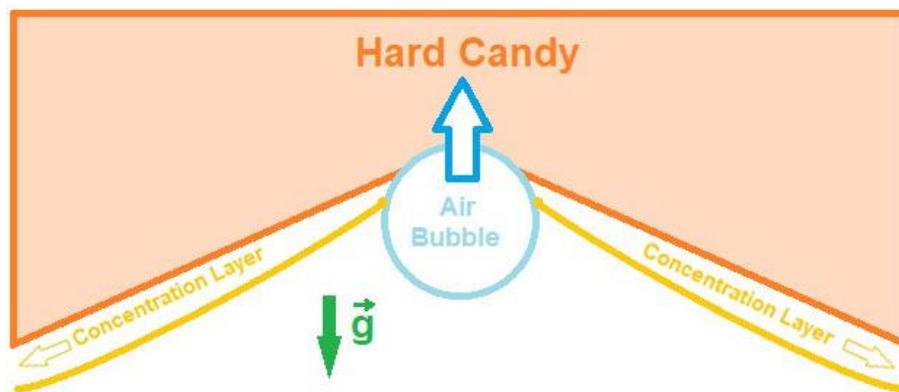
*Figure 59 Regression rate influenced by upward pushing bubbles.*
