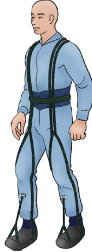
Figure 2.4: Penguin suit: the anti-zero-G suit looks like standard Russian in-flight suit, but had additional elastic band and pulleys that created a force against which the body need to work [6].
