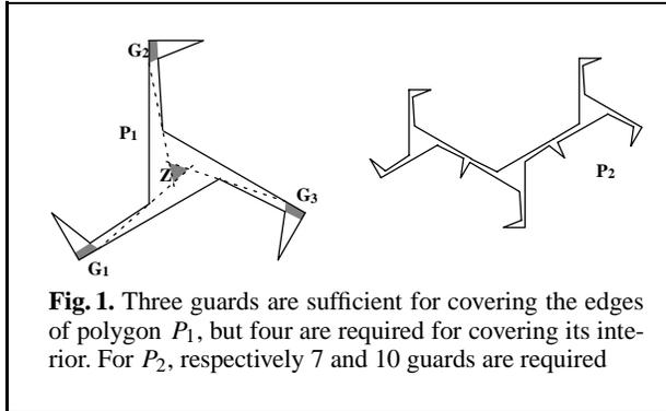
**Fig. 1.** Three guards are sufficient for covering the edges of polygon  $P_1$ , but four are required for covering its interior. For  $P_2$ , respectively 7 and 10 guards are required
