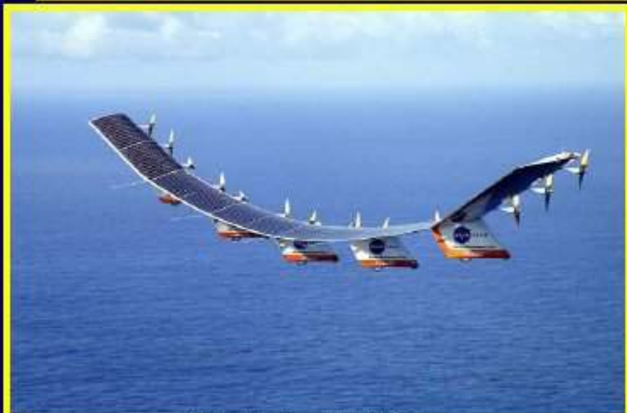
NASA Dryden Flight Research Center Photo Collection http://www.dfrc.nasa.gov/gallery/photo/index.html NASA Photo: EDD1-0209-2 Date: July 14, 2001 Photo by: Nick Galante/PWRF The Helios Prototype flying wing is shown over the Pacific Ocean during its first test flight on solar power from the U.S. Navy's Pacific Missile Range Facility.
