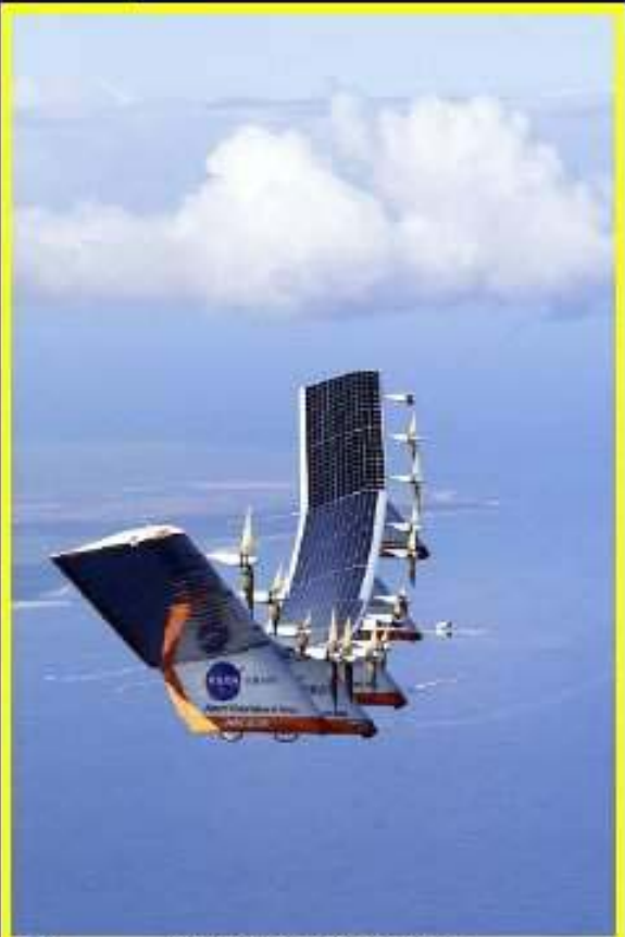
NASA Dryden Flight Research Center Photo Collection http://www.dfrc.nasa.gov/gallery/photo/index.html NASA Photo: EDD1-0209-2 Date: July 14, 2001 Photo by: Nick Galante/PWRF The Helios Prototype flying wing is shown over the Pacific Ocean during its first test flight on solar power from the U.S. Navy's Pacific Missile Range Facility.
