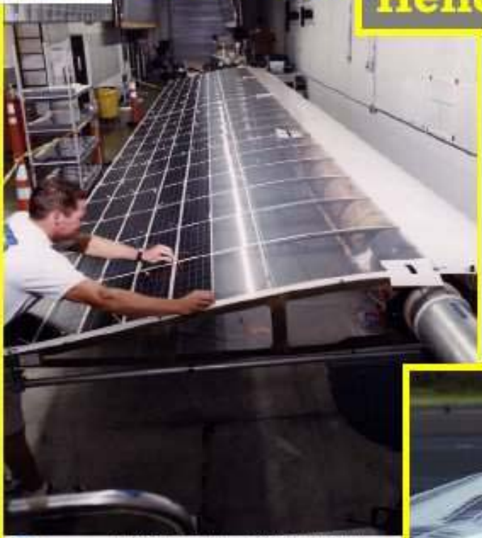
NASA Dryden Flight Research Center Photo Collection http://www.dfrc.nasa.gov/gallery/photos/index.html NASA Photo: EC00-0250-4 Date: September 16, 2000 Photo by: Tom T... Technician Marshall RibCready installs solar cells on the Helios Prototype
