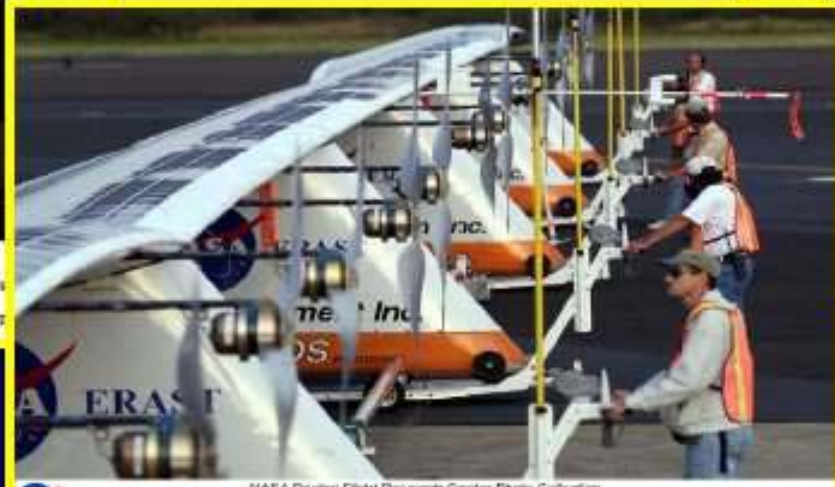
NASA Dryden Flight Research Center Photo Collection http://www.dfrc.nasa.gov/gallery/photos/index.html NASA Photo: EC01-0148-0 Date: April 28, 2001 Photo by: Nick Galante Ground crewman maneuver the Helios Prototype flying wing on its ground support dolly during functional checkouts prior to its first flight under solar power.
