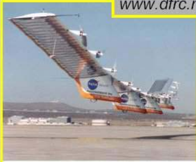
Dryden Flight Research Center - EC26-4180-127. Photographed NOV1998. The Centurion solar-electric flying wing, one of several remotely piloted aircraft being developed under NASA's ERAST program, flies toward a landing on Rogers Dry Lake. NASA/Dryden/Carl Thomas
