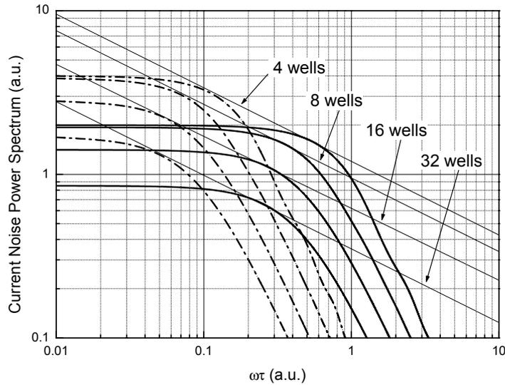
**Figure 4.** Power spectral densities of current noise obtained by numerical solution of Eqs.(7) and (8). The curves refer to  $N = 4, 8, 16, 32$  and to  $p_c = 0.35$ . Continuous lines and dashed lines differ for the characteristic time  $\tau$  used in the Fourier transform algorithm. It can be observed that a  $1/f$  slope is obtained by adding several noise components like the single Lorentzian curves plotted in this figure.
