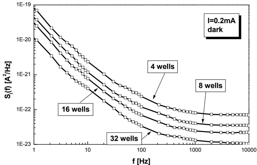
**Figure 1.** Power spectral densities of the current noise for AlGaAs/GaAs QWIPs respectively with  $N = 4, 8, 16, 32$ . All the curves refer to dark condition, temperature  $T = 90K$  and current  $I = 0.2mA$ . The noise spectra are  $1/f$ -like at low frequencies, while at the high frequencies become flatter. The  $1/N$ -dependence is almost rigorously respected all over the investigated range of frequencies.
