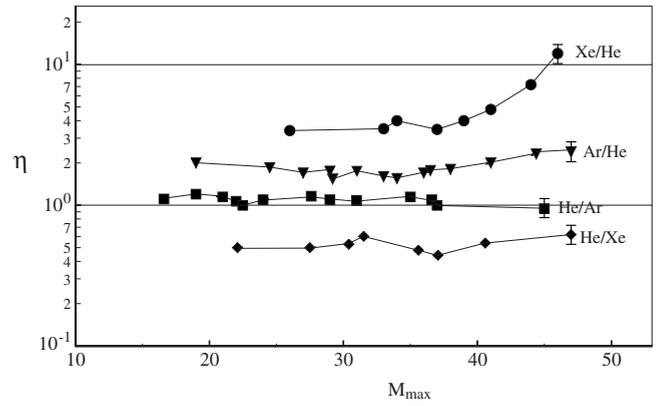
FIG. 8. Parameter domain  $M_{max}\eta$  (maximum Mach number—density ratio) of the tested jets. Sample error bars are shown on the right.
