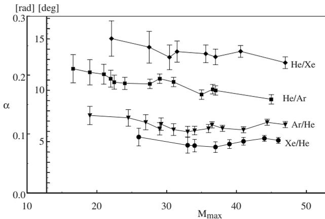
FIG. 10. Spreading angles of the plumes outside the barrel shock vs  $M_{max}$  for several jet/ambient gas pairs. The density ratio ranges are  $0.50 < \eta < 0.62$  for He/Xe,  $0.95 < \eta < 1.20$  for He/Ar,  $1.54 < \eta < 2.40$  for Ar/He and  $3.40 < \eta < 12.0$  for Xe/He.
