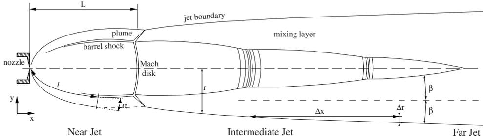
FIG. 2. Structure of a strongly underexpanded jet.  $L$  is the nozzle-Mach disk distance or barrel length,  $\alpha$  is the plume growth angle measured on an arc of length  $l$ ,  $r$  is the conventional jet radius, and  $\beta$  is the mixing layer spreading angle in the intermediate jet.
