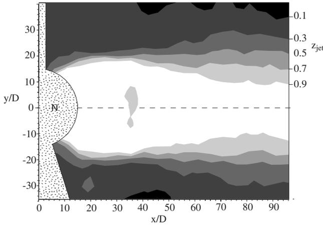
FIG. 7. Concentration map of the xenon jet visualized in Fig. 4. The zone marked with “N” cannot be analyzed, since the relevant pixels are in the density saturation range, fall outside the electron sheet, or are influenced by the nozzle image.
