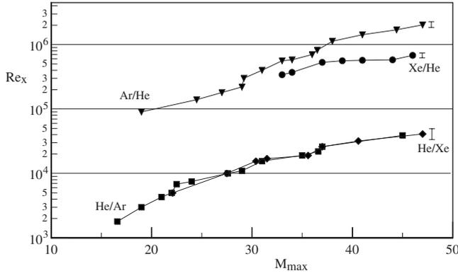
FIG. 9. Maximum longitudinal Reynolds number  $Re_x$  upstream from the Mach disk as a function of  $M_{max}$ . Sample error bars are shown on the right
