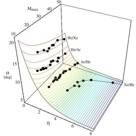
FIG. 11. (Color online) Scaling law Eq. (11) for the plume spreading angle as a function of the Mach number  $M_{max}$  and density ratio  $\eta$ .
