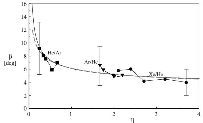
FIG. 12. Spreading angles of intermediate jets vs density ratio (the axial Mach number downstream from the Mach disk is about 0.45 for all the jets). The solid line is a fit according to Papanoschou and Roshko (1988) [13], the dashed line is the best scaling law fit, see formula (13).
