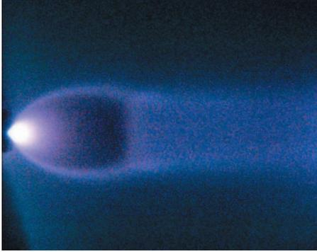
FIG. 4. (Color) Example: Xenon jet in a Helium medium. Pressure ratio  $p_0/p_{amb} \sim 4.3 \cdot 10^3$ , Mach before the normal shock  $\sim 41$ , Reynolds number at the nozzle exit  $= 2.5 \cdot 10^4$ .
