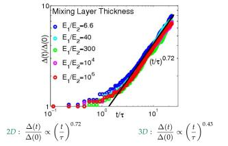
2D turbulent diffusion is infinitely grater than 3D diffusion: by defining a diffusion velocity as  $v_D = dx_s/dt = \eta d\Delta/dt$  we have  $v_D = \propto t^{-0.28}$   $v_D = \propto t^{-0.57}$
