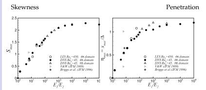
We define the penetration as the position of the maximum of the skewness normalized over the mixing layer thickness:  $\eta = \frac{x_s(t)}{\Delta(t)}$
