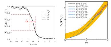
$\Delta(t)$  is the conventional mixing layer thickness,  $\Delta(t) \sim t^{0.46}$
