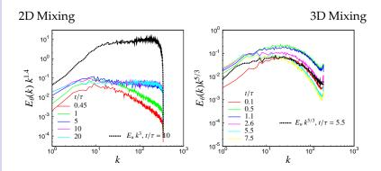
Compensated scalar and velocity one-dimensional spectra in the same position
