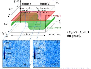
2D Velocity stati Uniform kinetic energy Passive scalar Mean Scalar
