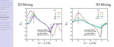
Strong non-gaussian statistic at the mixing layer border 2D: intermittency penetrates more in the direction opposite to the energy gradient.
