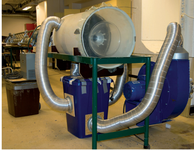
FIGURE 3.3. Inlet section of the pipe flow facility
