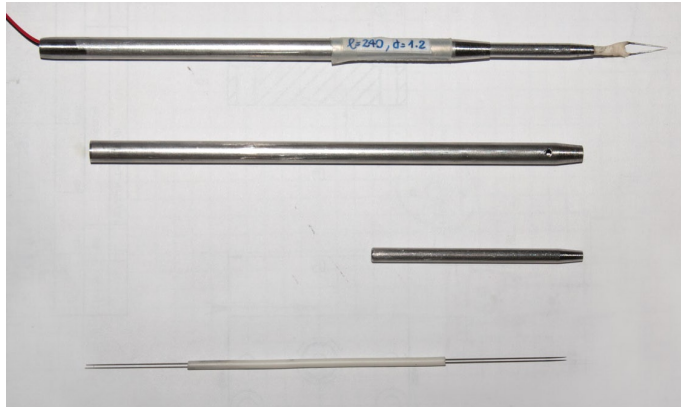
FIGURE 3.17. Probe's components together with a finished probe ( top ).
